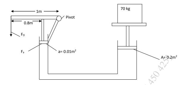
If A and a are areas of cross-sections of the pistons and the lengths of the arm are as given. Find a) (i) the value of force  $F_0$  (4 marks)
