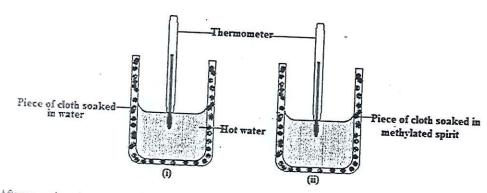
After some time, the thermometer in (ii) recorded a lower temperature. Explain this observation (2 marks) Methylated spirit evaporates faster than water; hence it takes away heat from the hot water faster than water.
