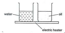
The specific heat capacity of water is higher than that of oil. State with a reason the liquid that will have a higher temperature after one minute (2 marks)
