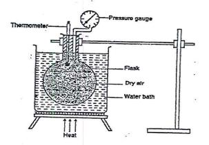
State with a reason which gas law is being experimented by the set-up
