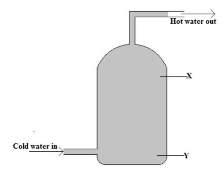
State with a reason whether the appropriate position for a heater is X or Y(2 marks)**Position Y. To ensure heat is transferred upwardly in the water through convection**
