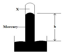
State and explain the effect on the height h when the atmospheric pressure increases (2 marks) <u>The height increases</u>. Increase in atmospheric pressure will push the level of the mercury column to rise in the tube
