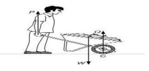
There are three vertical forces acting on the wheelbarrow P is the upward force applied by the gardener. Q is the upward force of the ground on the wheel at point C.W is the weight of the wheelbarrow and its contents. Explain why the force P is less than the force W
