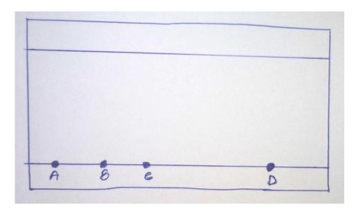
After development A, B and C were found to have moved 4cm, 1.5cm and 3cm respectively. D has separated into two spots which had moved 3cm and 4cm.
