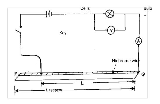
ii) With the crocodile clip at P take the voltmeter reading and the ammeter reading. Record V and I. Repeat the readings for L = 80,60,40,20 and 0 cm respectively. Complete the table below;
