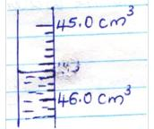
the 0cm<sup>3</sup> mark. The figure shows a burette showing the level of the liquid the liquid had been run out.
