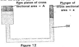
When the plunger moves down a distance d the Ram piston moves up a distance D.
