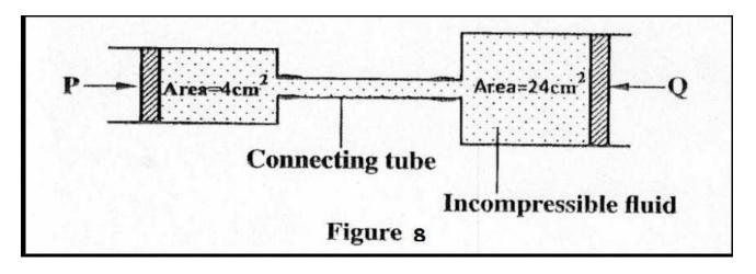
Opposing forces P and Q are applied to the pistons such that the pistons do not move. If the pressure on the smaller piston is 5 N cm 2, Determine force Q. (2 marks)
