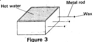
What property of metals could be tested using this set-up? (1mk)
