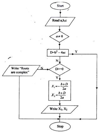
b) Using the flow-chart write a program that will compute the roots and if  $b^2$  – 4ac is negative, the program should display the message "NEGATIVE" (5mks)
