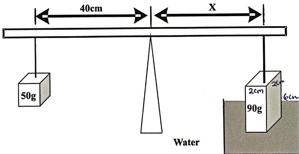
(i) When the temperature of the water is raised, the system is observed to tilt to the right. State the reason for this observation. (2mks)
