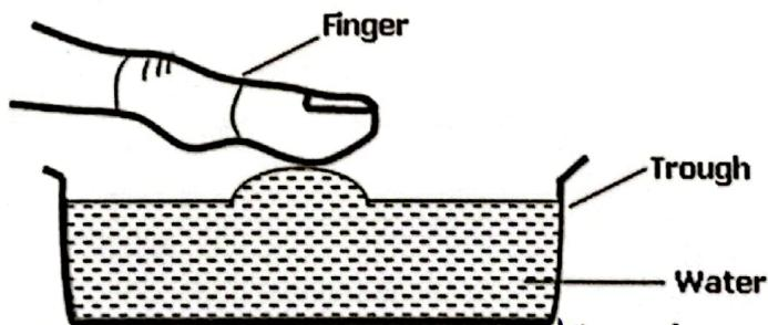
Name the force that lifts the water to the finger. Adhesive force ✓ 1 (1mk)
