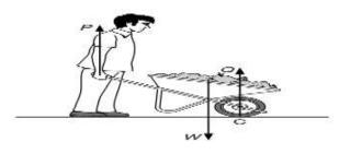
There are three vertical forces acting on the wheelbarrow P is the upward force applied by the gardener. Q is the upward force of the ground on the wheel at point C.W is the weight of the wheelbarrow and its contents. Explain why the force P is less than the force W
