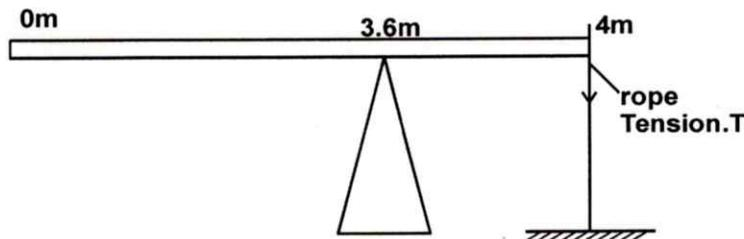
Calculate the tension, T in the rope (Take  $g = 10\text{N/kg}$ ) (3 marks)
