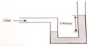
If a mercury barometer reads 760mm, calculate the pressure of gas (give your answer in N/m<sup>2</sup>).
