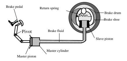
The brake drum rotates with the wheel of the car.
