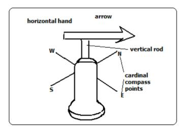
Wind direction is determined using wind vane.
