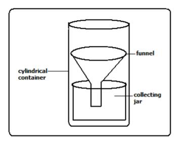
Rain gauge is the instrument used to measure the amount of rainfall in a day.
