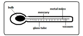
It's used to measure the highest temperature reached in a day.
