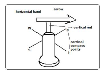
Wind direction is determined using wind vane.
