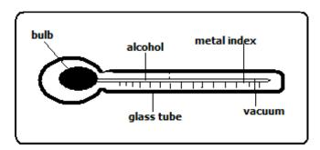
It's used to record the lowest temperature reached in a day.
