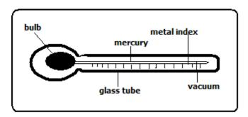
It's used to measure the highest temperature reached in a day.
