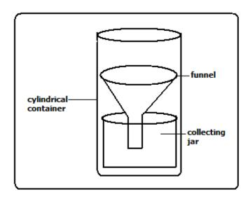
Rain gauge is the instrument used to measure the amount of rainfall in a day. It should be made of impermeable material which can't absorb water.
