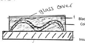
8. The figure (2) below shows a section of a solar heater
