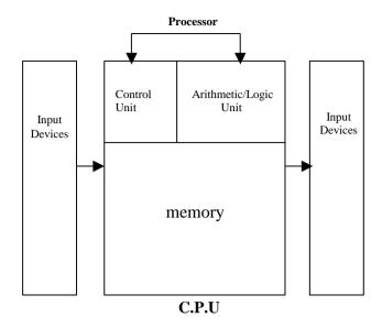
Fig. 2.5: Components of a Computer Hardware System
